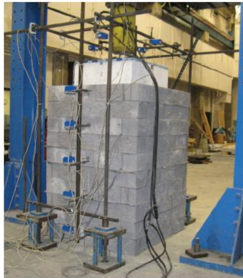
Faced GRS Mini-Pier (Nicks et. al, 2013)
