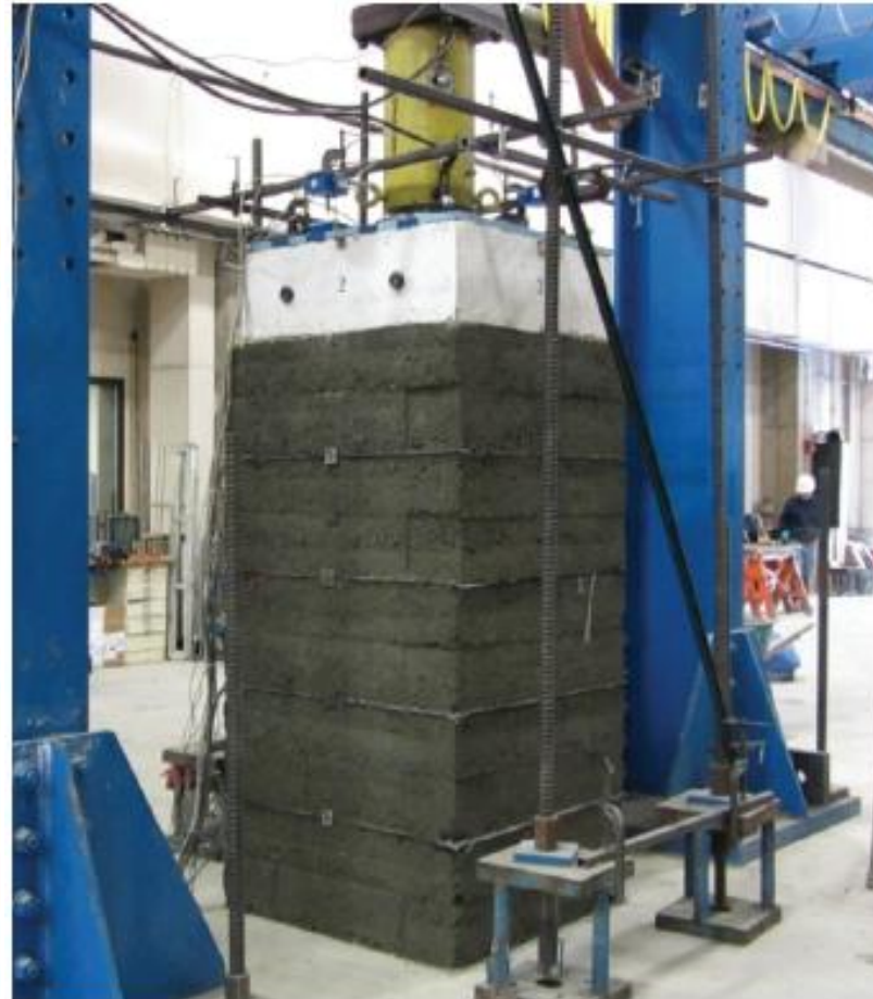
Unfaced GRS Mini-Pier (Nicks et. al, 2013)
